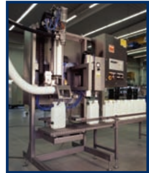
Container filling station type 14. Flexible solution which enables the filling of different container types due to low resetting work.
