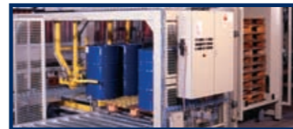
Automatic drum filler type 86. 216 l-drums are processed in six working stations from debunging and filling to safe bunging with an output of up to 120 drums per hour.
