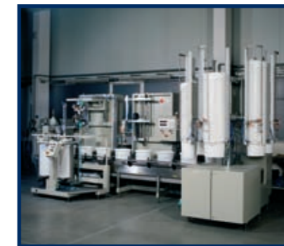
Container filling equipment type 24. Semi automatic filler, here in stainless steel equipped with a semi automatic bunging station.
