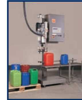
Container filling station type 14. Flexible solution which enables the filling of different container types due to low resetting work.
