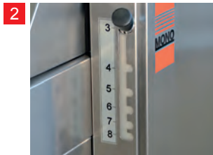
Sheeting Roll Gap Dough rolled thickness can be quickly changed using the easily adjustable controls.
