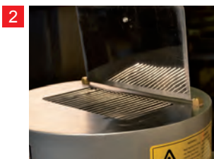
Flour Duster The integral flour duster, with variable output, can be used to prevent dough sticking.
