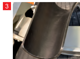
Teflon Coated The cone and off-take chute are both teflon coated which prevents dough from sticking.
