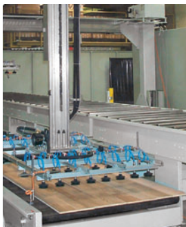
STACKING | FEEDING: A production cycle often starts or ends with the automated feeding or removing of parts. The illustrated feeding or stacking equipment is equipped with transverse vacuum suction, for installation in pit or pitless design.
