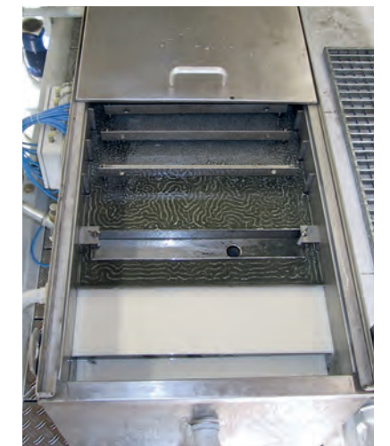
Coalescers for separation of a light liquid secondary phase from a liquid main phase, e.g. tramp oil from wash water
