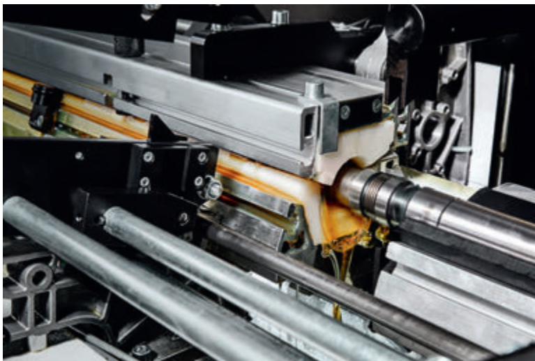
Optimum guidance Oil-flushed guide channel with hydrodynamic bearing effect
