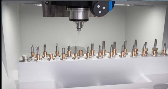
24-station tool magazine with integrated tool-length sensor
