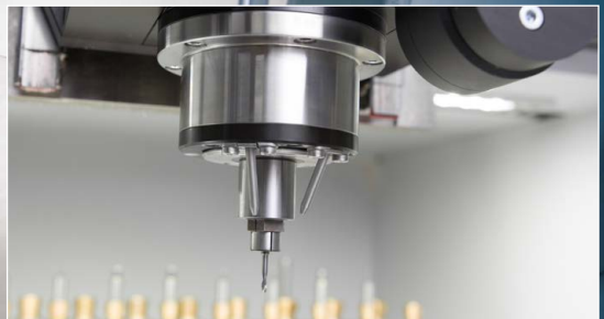
2 kW spindle and minimum-quantity coolant system
