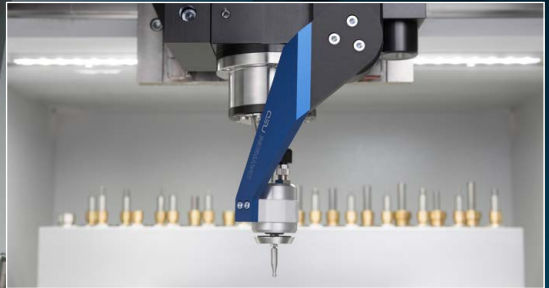
3D probe (XYZ sensor) and camera
