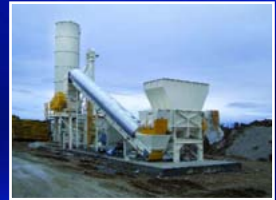
Plant for recycling of gas-/cellular concrete scrap
