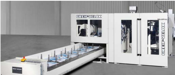
High-performance machine for automatic placing of pre-made empty bags
