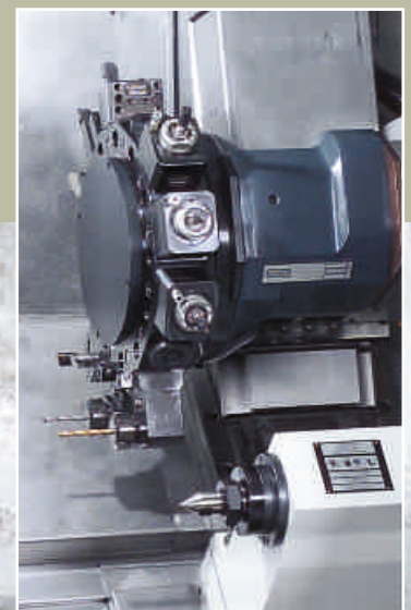
Y axis fully integrated in the machine bed
