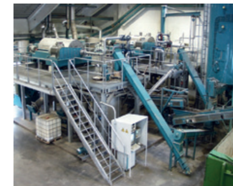
▲ Two-stage CENSOR installation for sorting mixed plastics: absolutely pure PA granulate
