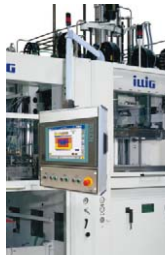
Operating panel UA-g machines. Digitized functions enable computer-aided basic setting of the machine data.
