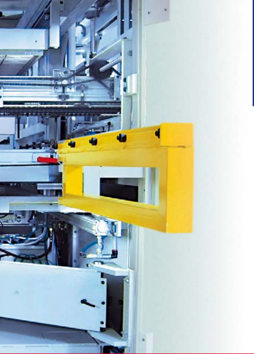
Higher output potential by application of pre-heating and off-station technology in the sheet loading device
