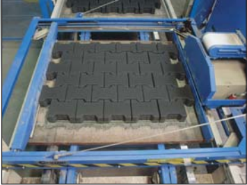
Horizontal strapping of paving blocks
