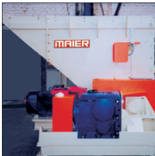
Large volume material hopper with external shaft bearing and gear.
