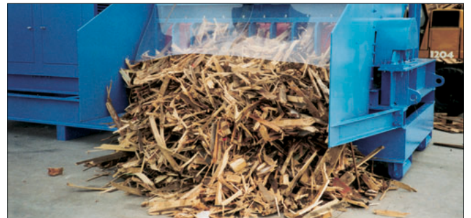
Pre-crushed material at the discharge grate of the MGB.
