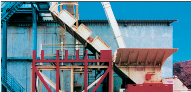
MGB 132/3000 with hydraulic dosing table for automatic feeding with PB, MDF, OSB boards.
