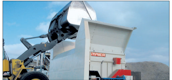
Feeding of the MGB with a bucket-wheel loader.
