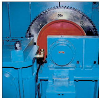
Large wheel with shearing bolt to protect the gear in the event of a sudden blockage.
