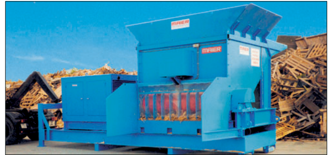
Semi-mobile MGB with diesel generator for use on different sites.
