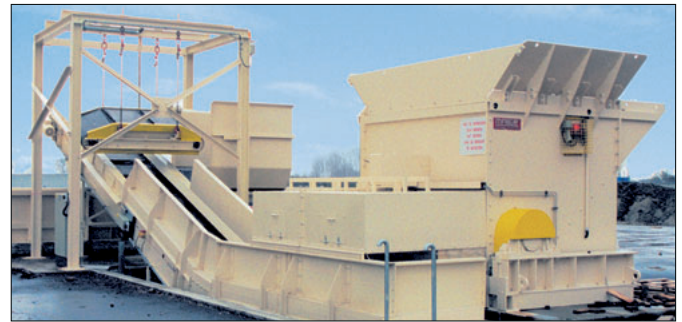
MGB crusher 132/3000 with discharge belt and overband magnet assembled to form a complete plant.
