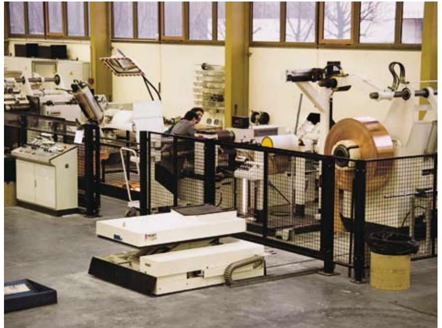
Kupfer, Messing, Bronze, Aluminium copper, brass, bronze, aluminium 0,05-1,5mm x 400mm 300 m/min
