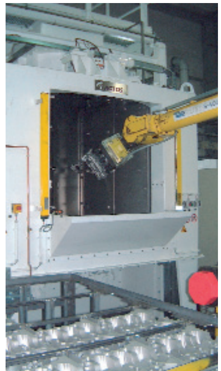
Automated satellite turntable blast machine for castings.
