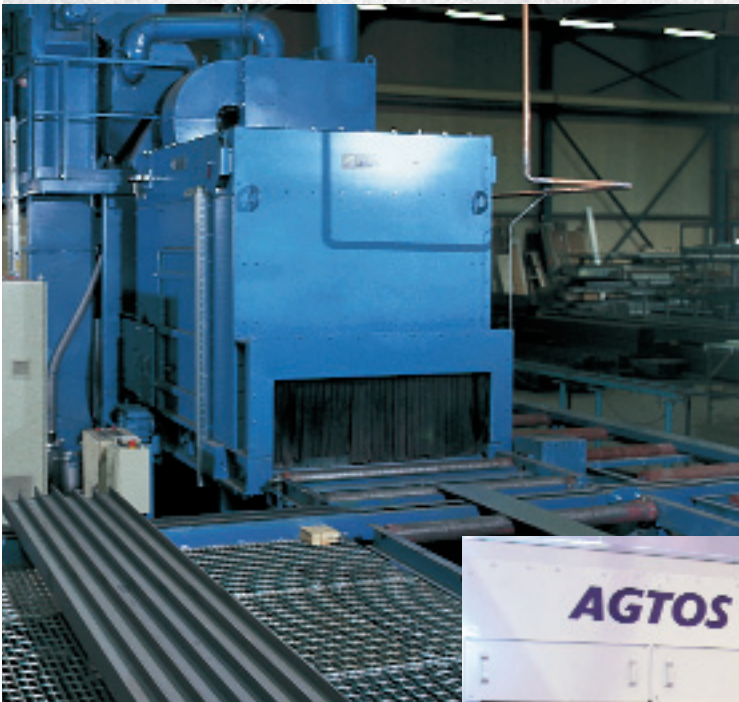
Roller conveyor blast machine with crossover conveyor technology.
