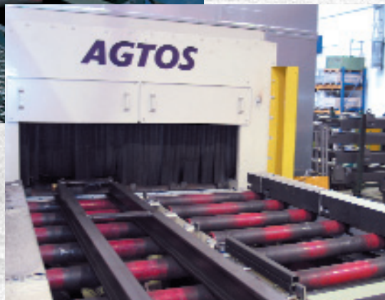
Roller conveyor blast unit with oversized passageway for blasting machine constructions.
