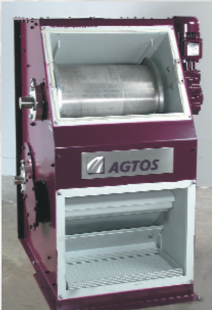
Retrofitting of blasting machines with magnetic air classifiers for the separation of abrasive and sand.
