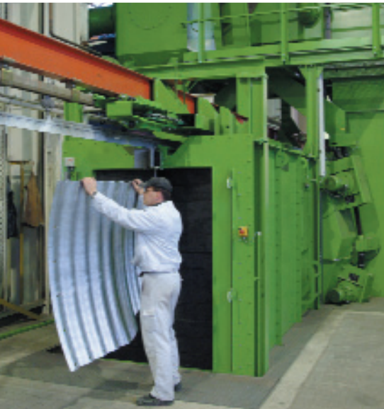
Hanger-type blast machines are engineered as stand-alone solutions or designed for applications requiring continuous operation.
