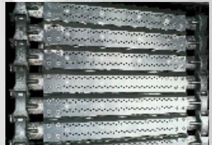
Configuration of steel mill tumble blast machines with new wear-parts.
