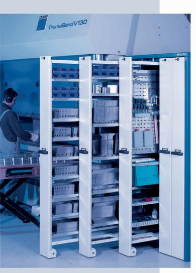
Reduce set-up times through a well-arranged tool storage in the vertical drawers of our WKS series.
