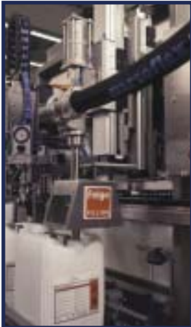
Filling station, below-surface with gas hood
