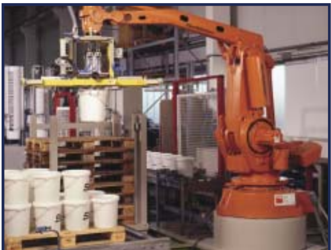
The pails are palletised by the robot as per pre-set pallet scheme.
