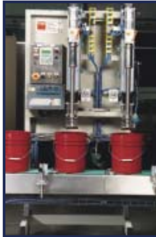
Double filling station below-surface
