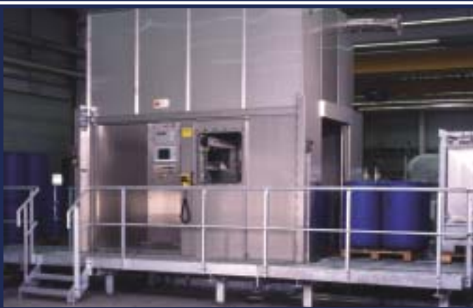
Pallet filling robot Type 71. here in enclosed housing made of stainless steel with sliding doors in the in-feed and out-feed area.
