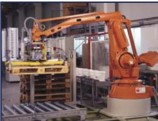
Palletising robot with combination tools The robot takes a pallet out of the magazine and places it on the out-feed conveyor.
