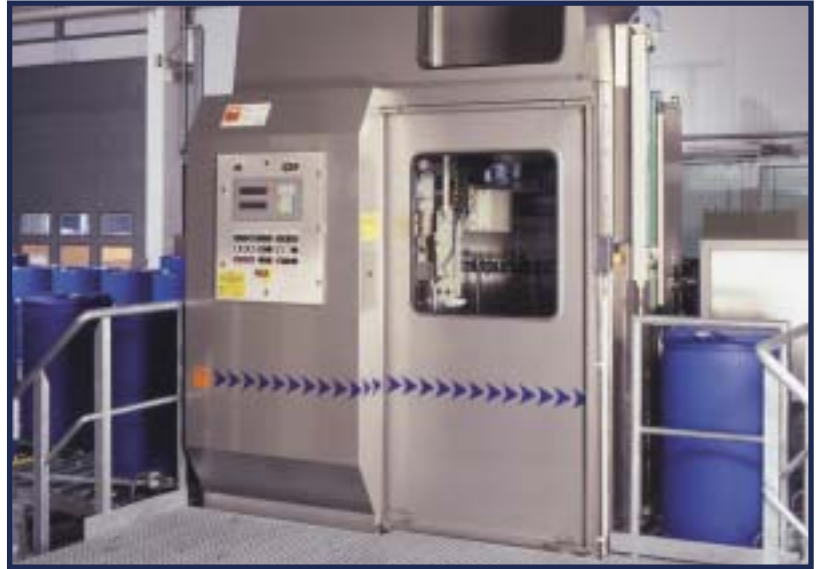
Your drum is automatically positioned, debunged, filled, bunged and sealed. Drum filler Type 81.
