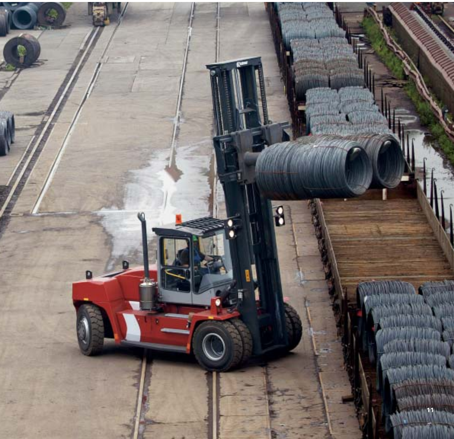
Custom-built machines with special attachments make work efficient and problem-free. The cab is high with large glass areas for the optimum visibility.
