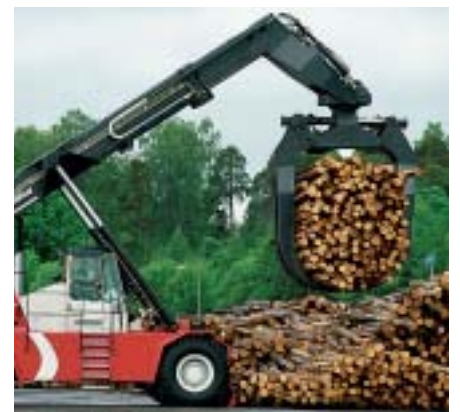
The log handler has been specially developed to handle timber, and can unload an entire trailer in one lift.
