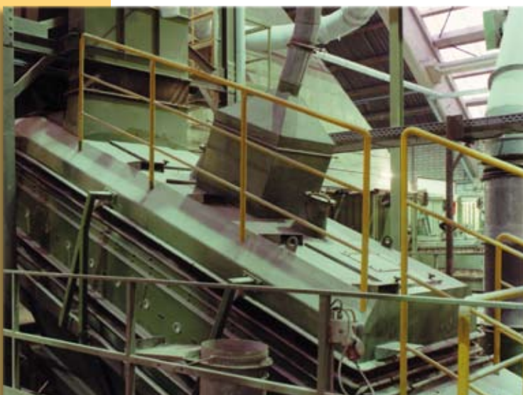
LL 1.5-5.04 / 24 ED - 7.5 m 2 for recycling of packaging material. Separation at 10 mm. Feed capacity of 60 m 3 /h.
