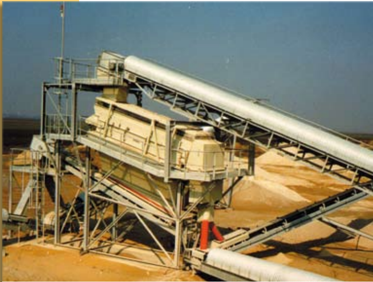
LF 2.0-6.30 / 20 DD - 25 m 2 for crushed stone fines. Separation at 5 mm and 2 mm. Feed capacity of 200 t/h.
