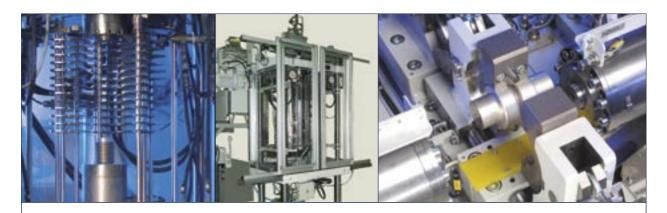
The metal bellows are made from straight tubes by means of an internal hydraulic pressure and a simultaneous compression. Modular tools or special tools for two chamber bellows are used as forming instrument.
