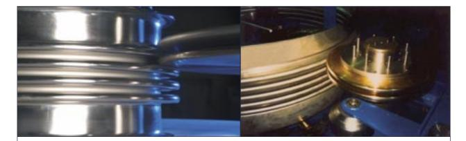
Mechanical Roll Forming Machines are used for the production of large diameter metal bellows from multiple welded tubes by the single convolution forming principle.
