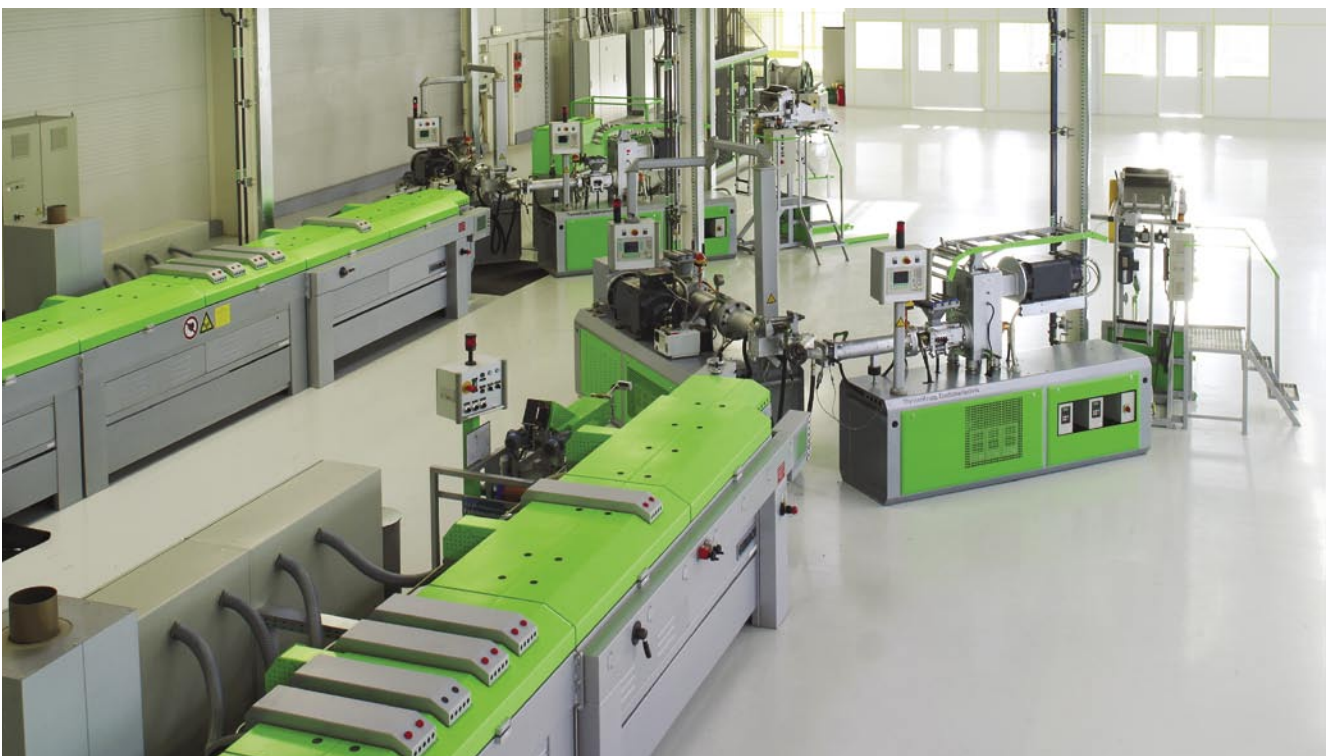
Extrusion line for the production of profiles for the automotive industry
