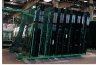
xx Rack stillages – Substrate glass, front glass and photovoltaik panel storage – Heat- and pressure resistance for autoclave with spacers
