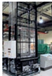
xx Storages and Accumulator – FiFo or LiFo principle – Up to 100 glass sheets capacity – Cooling opportunity – Horizontal and vertical systems
