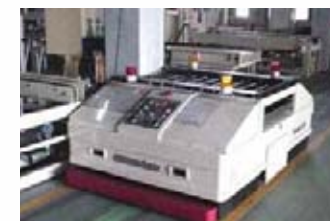
xx AGV Shuttle – Enables access to processing equipment for service and maintenance – Transport of single / multiple substrates – Cassette transportation
