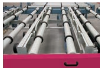
xx Roller- / Roller angle transfer conveyor – Reduced maintenance conveying technology
