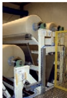
xx PVB foil applicator – Handling up to 4 PVB coils – Bumper rolls for PVB foil relaxation and buffer with feedback to coil unwinder speed – Rotating knife – Puncher – Seamless foil connection
