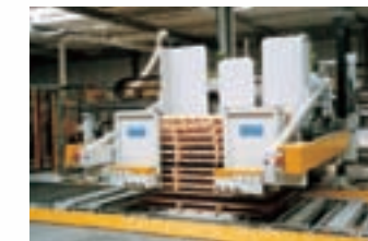
xx Automated palett feeder/ module sorting – Automated packing – Different orientation (horizontal and vertical)
