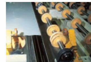
xx PVB foil trimming – Trimming of foil rests – Rejection of trims – Trimming on 4 sides – Combination with conveying technology
