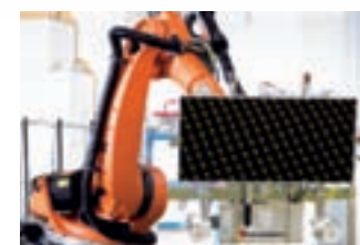
xx Robot handling – De-stacking from substrate back side and loading on conveyor – Landscape or portrait – Spacer removal – Interleaver paper removal and elimination
