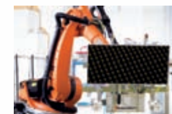
xx Robot handling – Stacking from substrate back side or front side, landscape or portrait – Spacer application – Simulator handling
