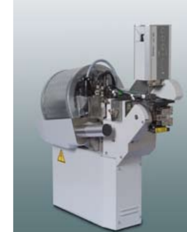
mci 765 seal loading module with seal position monitoring (SPM)
