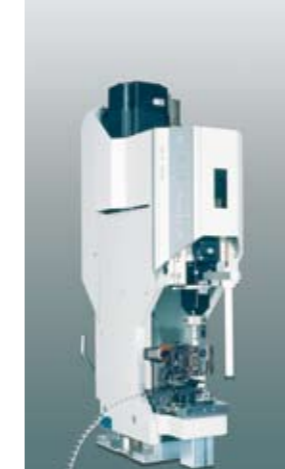
mci 722 crimping module with programmable crimp height
