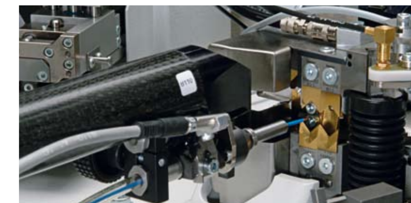
Blade head (dual-channel blade system)
