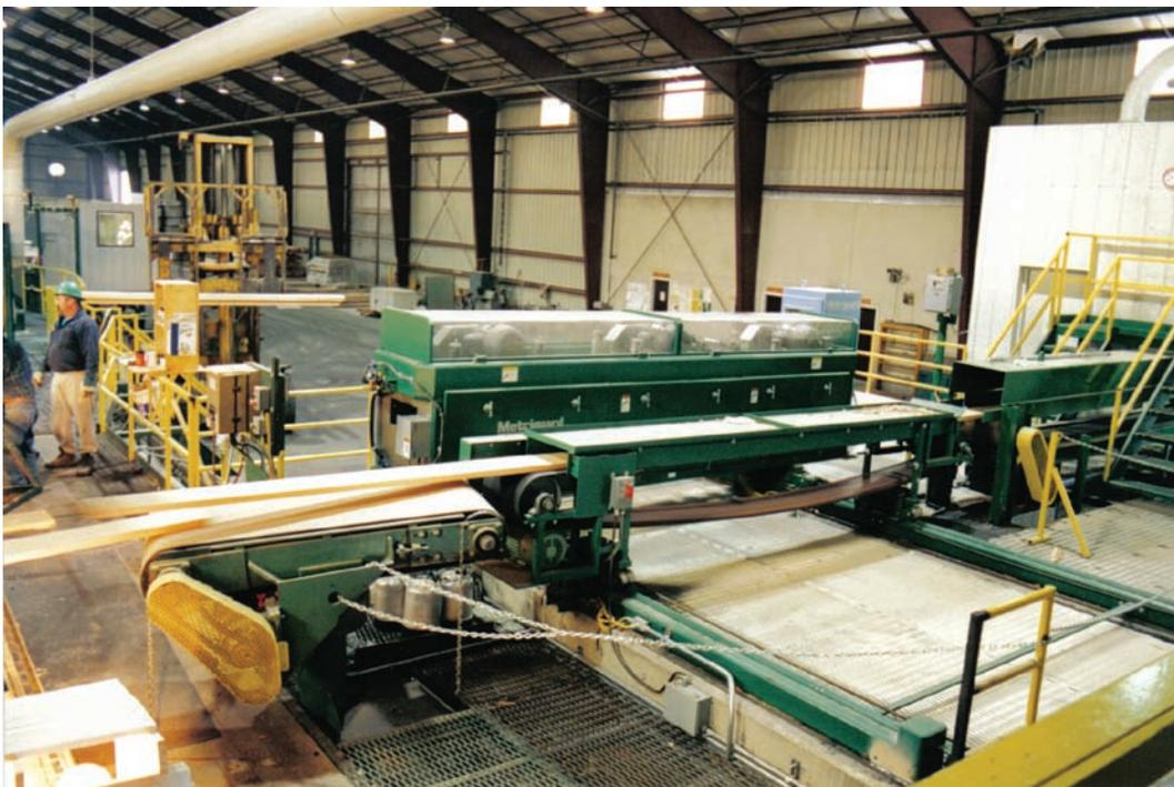
View of a Model 7200 HCLT and bypass conveyor on a shifting base, showing the bypass conveyor in line and the 7200 shifted offline.
