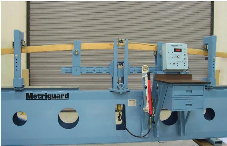
Model 312 Bending Proof Tester shown here measuring modulus of rupture (MOR) by taking a 2x4 to failure.
