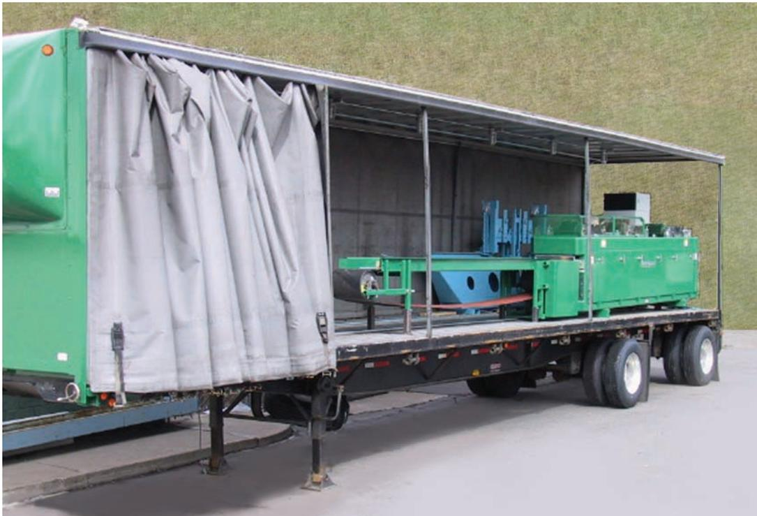
The Metriguard Mobile MSR Unit includes a Model 7200HCLT with PC Data System, plus a Model 312 Bending Proof Tester, infeed conveyor, and landing table. The entire mobile unit is self-contained and powered by its own generator, requiring only a level parking lot area to stage and run.
