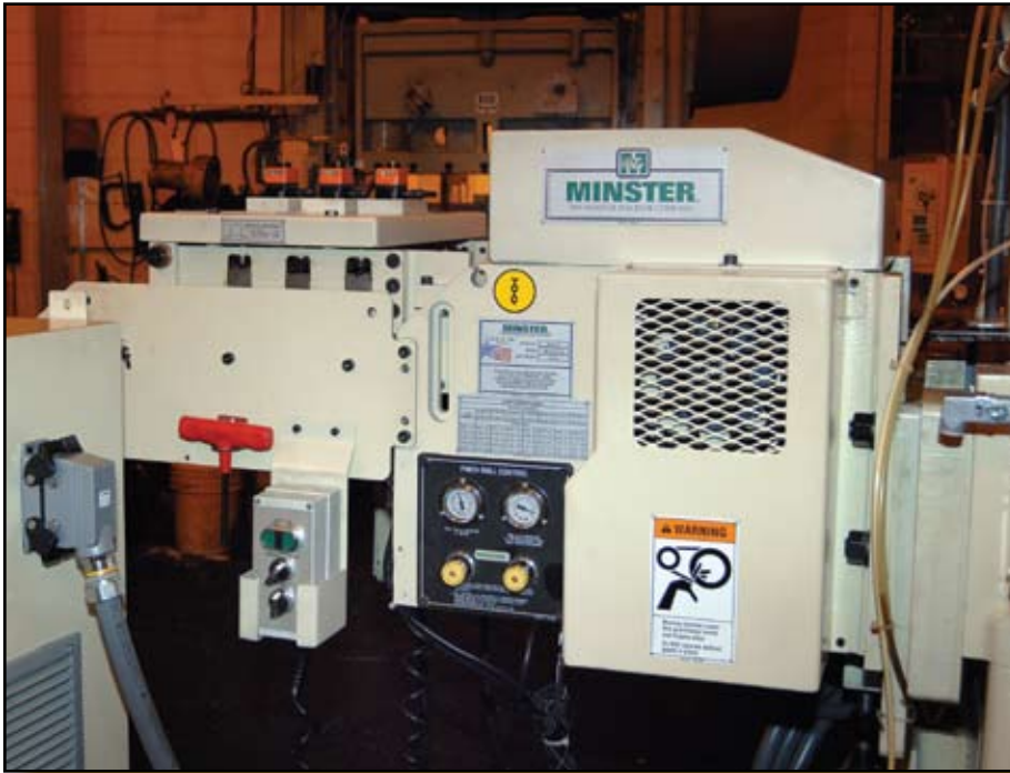
The Minster MEF2-CS Feed with Pull Thru Straightener at Allied Tool and Die rates at a maximum roll lift rate of 425 strokes per minute.
