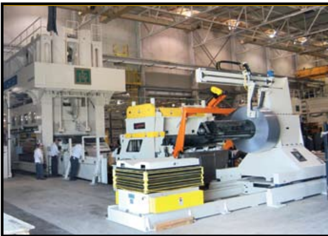
E4H feed line includes Machine Concepts straightener.
