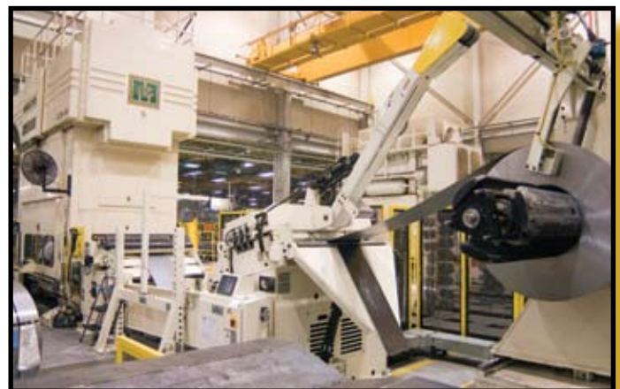
Minster feed lines assist in rapid job change-overs at KMI.
