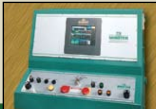
Full-Featured Minster Production Management Control incorporates all press functions.
