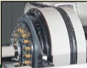
Patented Hydraulic Clutch & Brake for maximum torque and faster starting and stopping.
