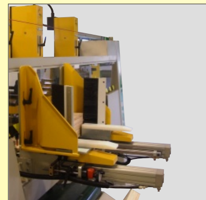
Components are fed in, held in position and ejected by pneumatic clamps, thus ensuring positive feeding without marking the timber.
