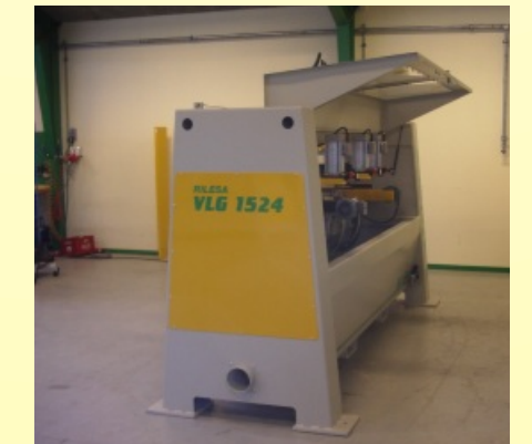
The machine is equipped with a large door on the backside, it gives easy access to the drilling groups.
