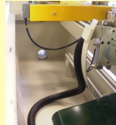
Dust extraction is integrated into the base of the machine.
