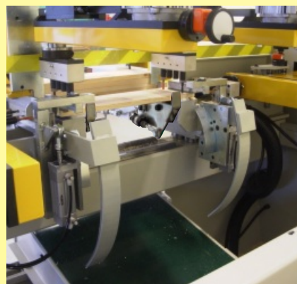
After drilling, the components are pushed through the skid down to the conveyor belt.
