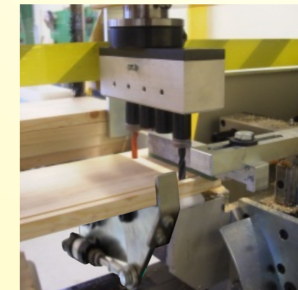
Combination of restraint, side pressure and top clamp cylinders hold the workpiece securely. This ensures optimum precision whilst drilling.
