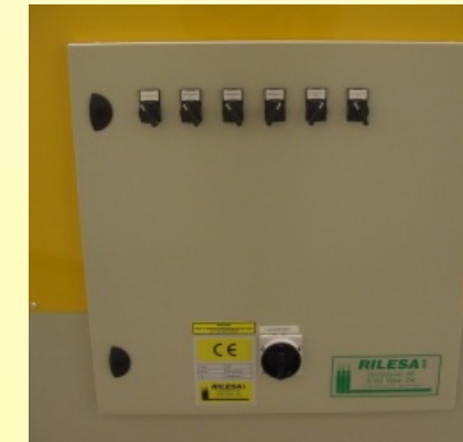
The control system is easy to operate. Each drill group, and the option cross drilling, is set by activating the switches.
