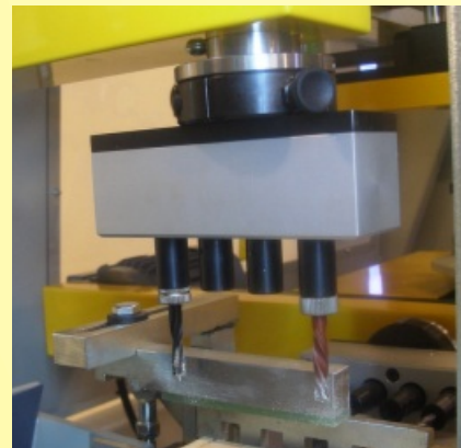
Assembly of drill boxes takes place with a snap function and is simply locked with screw. The drill box can be freely turned between 0 and 90°. In the outer positions there are stops.
