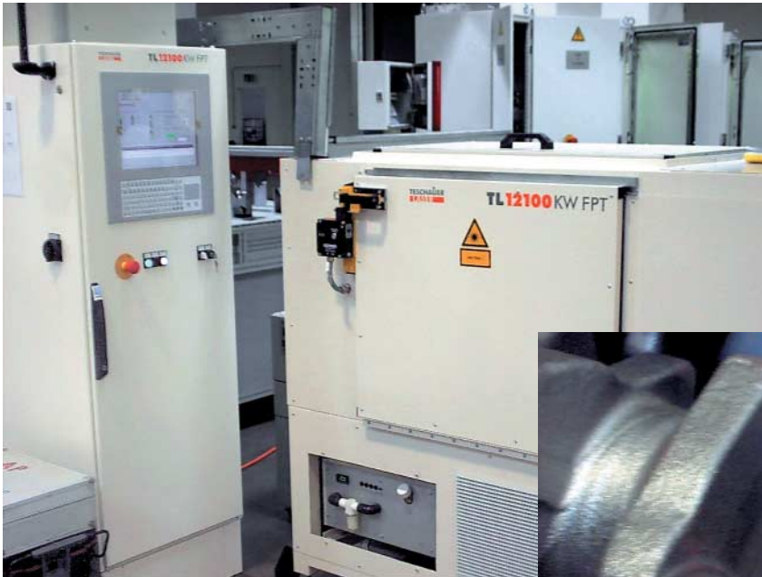
Special machine for laser marking – station of a flexible manufacturing line for crankshafts
