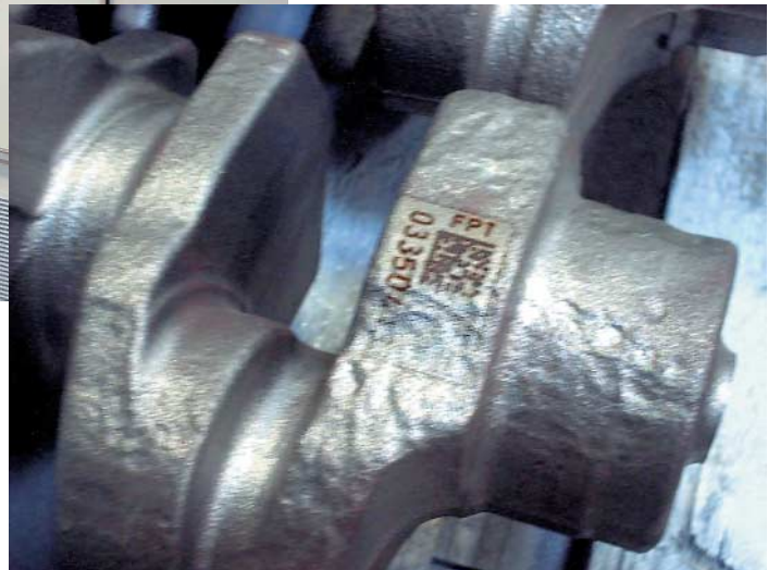
Special machine for laser marking – station of a flexible manufacturing line for crankshafts
