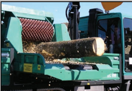
Feeder with active steel conveyor.
