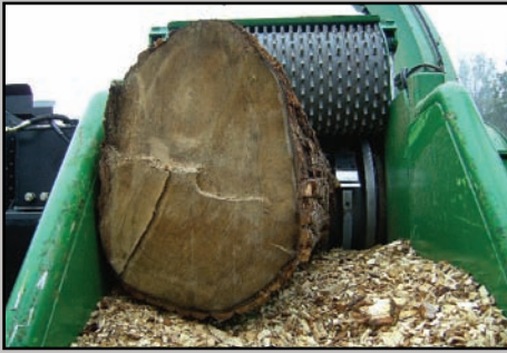
Patented segment construction of rotor:
