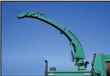
Pivoting supercharger with replaceable wearing parts. Optionally blowing functions via radio control.
