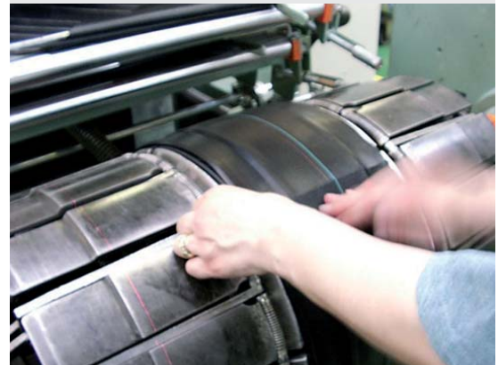
Tire building machine Z5-24F or Z5-24G
