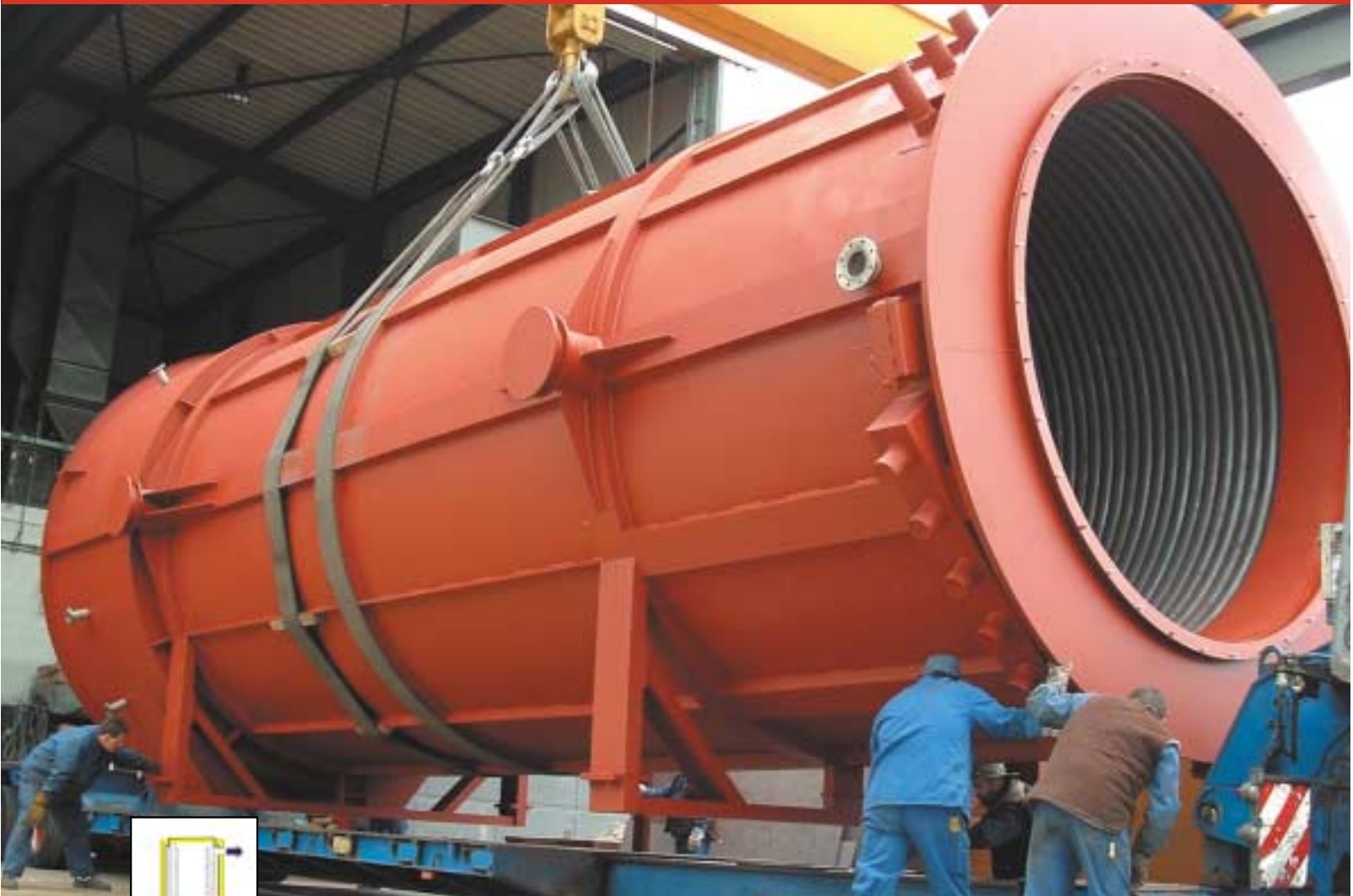
KONTAKTOMAT® - Solid Fuel fired Heater with intergrated sootblowers
