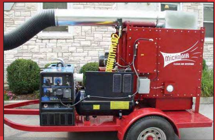
Trailer mounted RP4 collects cement dust
