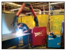
TM1000 Portable Collector in Weld Cell
