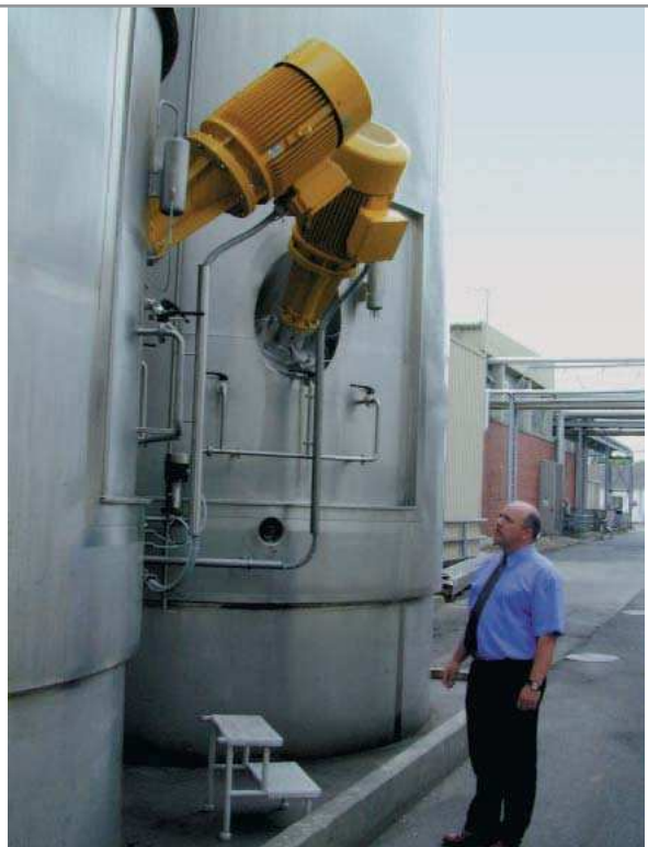
YTRON -Y in Side Entry Tank-flange execution below Liquid Level Application: Fermented Milk for Fromage Frais Production (100.000 litres capacity)
