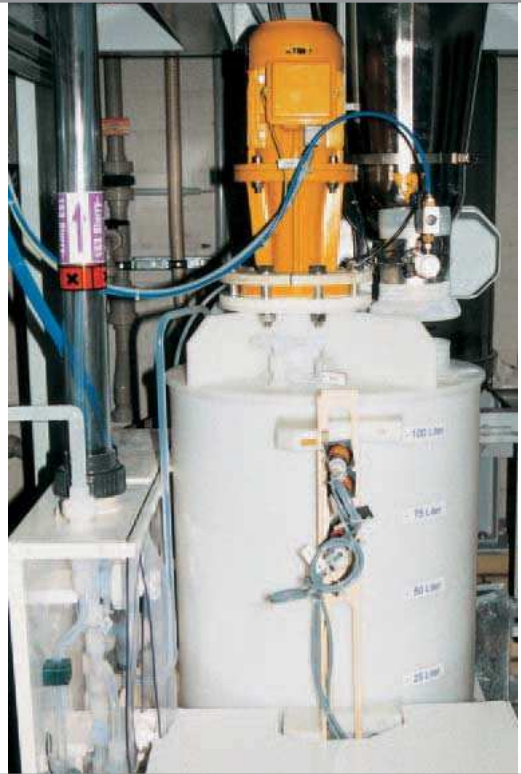
YTRON -Y installed on mating Flange of an Open Container Application: Suspension of Abrasive Polish
