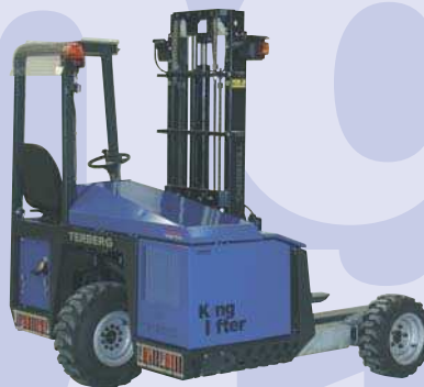
Model M is optionally available as a 4-way system, and also obtainable with retractable front wheels
