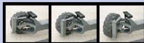
The 4-way steering system transforms the truck mounted forklift into an advanced side loader.
