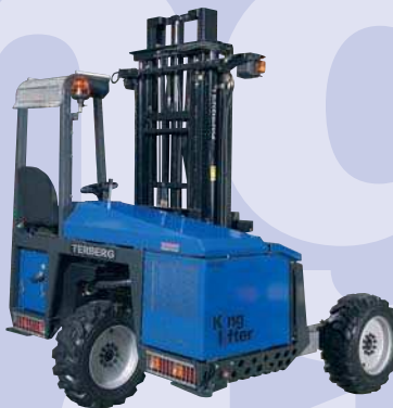
Model L is optionally available as a 4-way system, and also obtainable with retractable front wheels
