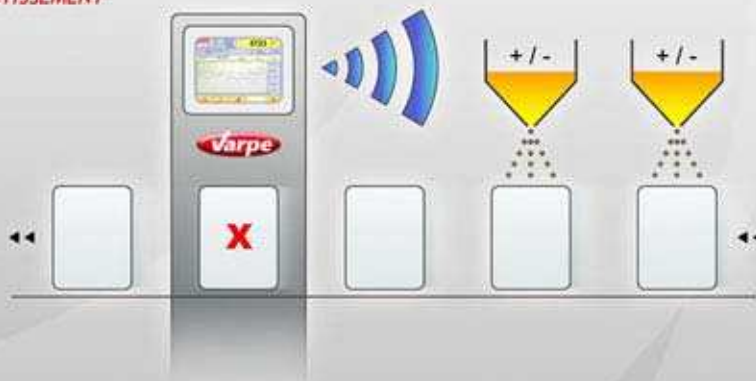
FEED-BACK: P.I.D. SYSTEM (Proporcional, Integral, Diferencial)
