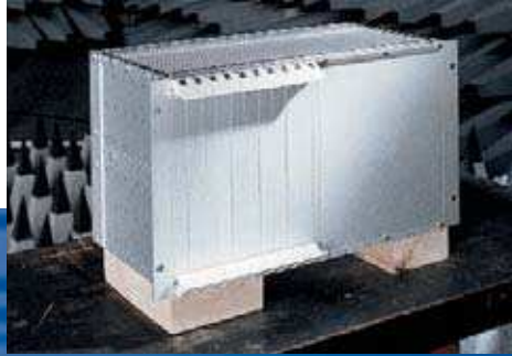
Subrack electromagnetic shielding performance test
