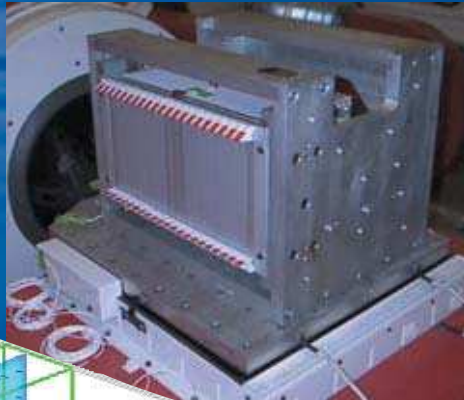
Subrack shock and vibration test
