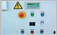
Stored-program controller PLC, operator panel with display.
