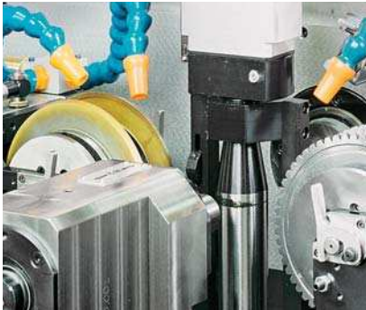
Chamfering/deburring unit with two self-centring tool heads for one tool group each
