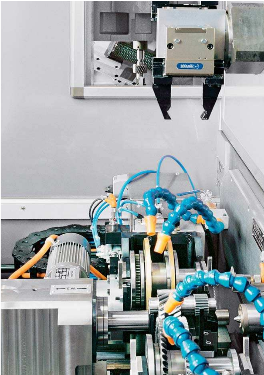
The integrated gantry loader transports the workpiece from the work area of the hobbing machine to the chamfering/deburring unit and further on to pass it on to the appropriate automated system
