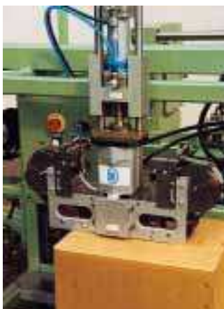
LRW-T twin stapling head for top stapling filled folding boxes. With adapter plate and conveyance cylinder.
