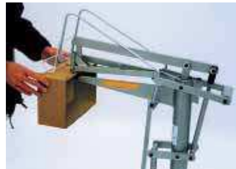
ST QE 270 P twin heads. 70 mm staple clearance. Two staple operations simultaneously.
