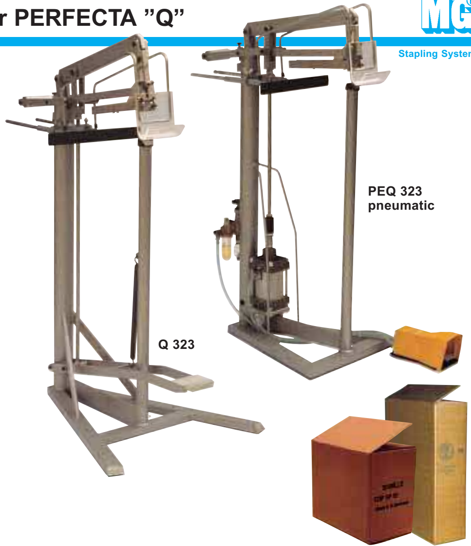
PEQ 323 Transversally mounted stapling head and a rapidly adjustable carton guide stop permit precise stapling parallel to the edge of the box.
