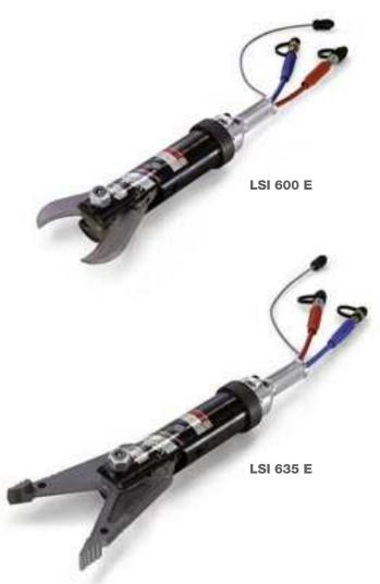
Extremely durable cutters designed with steel cylinder bodies for use in hostile environments with a high, cut frequency. The tools are push button operated. A solenoid valve on the power unit controls the opening and closing functions.
