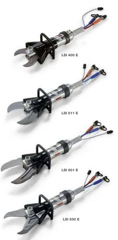
Powerful cutting tools with aluminum cylinder body design, combine to provide portability in a tool for applications requiring high cut frequency. The tool is push button operated. A solenoid valve on the power unit controls the opening and closing functions.
