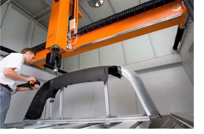
A laser beam which a gantry system guides in X, Y and Z directions, processes five sides of the part. In addition, the cutting head can rotate and swivel (A and C axes), which allows 6-side processing to some extent. The laser beam generates a programmed cutting contour in the part, which is clamped to a specific fixture and does not move during processing. Cutting heads with very small diameter are available for areas to which access is difficult or for recessed cuts.
