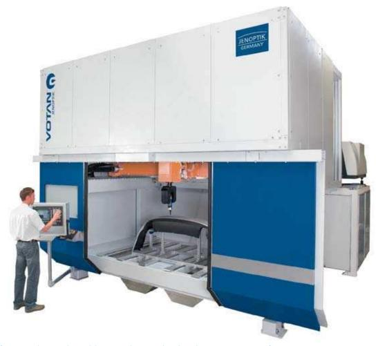
Much room for your application. The modular system design can be adapted to part sizes in steps of 10 cm. Thus, the part size is nearly unbounded.
