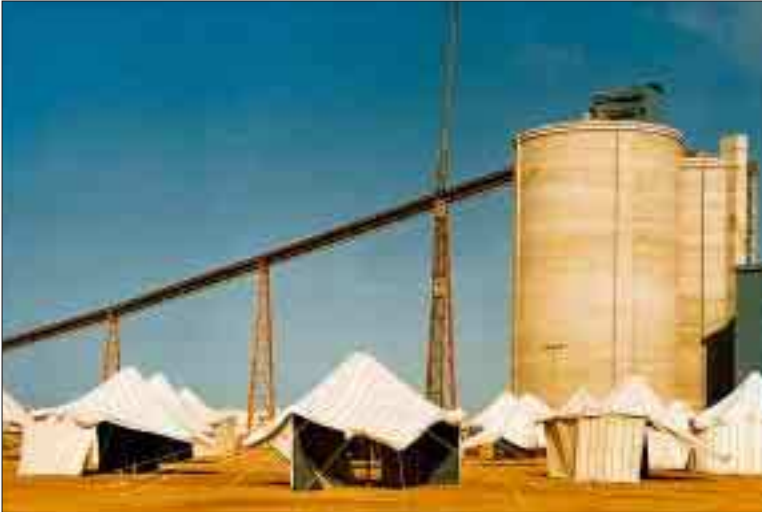
Ascending troughed belt conveyor for the feeding of a cement loading installation
