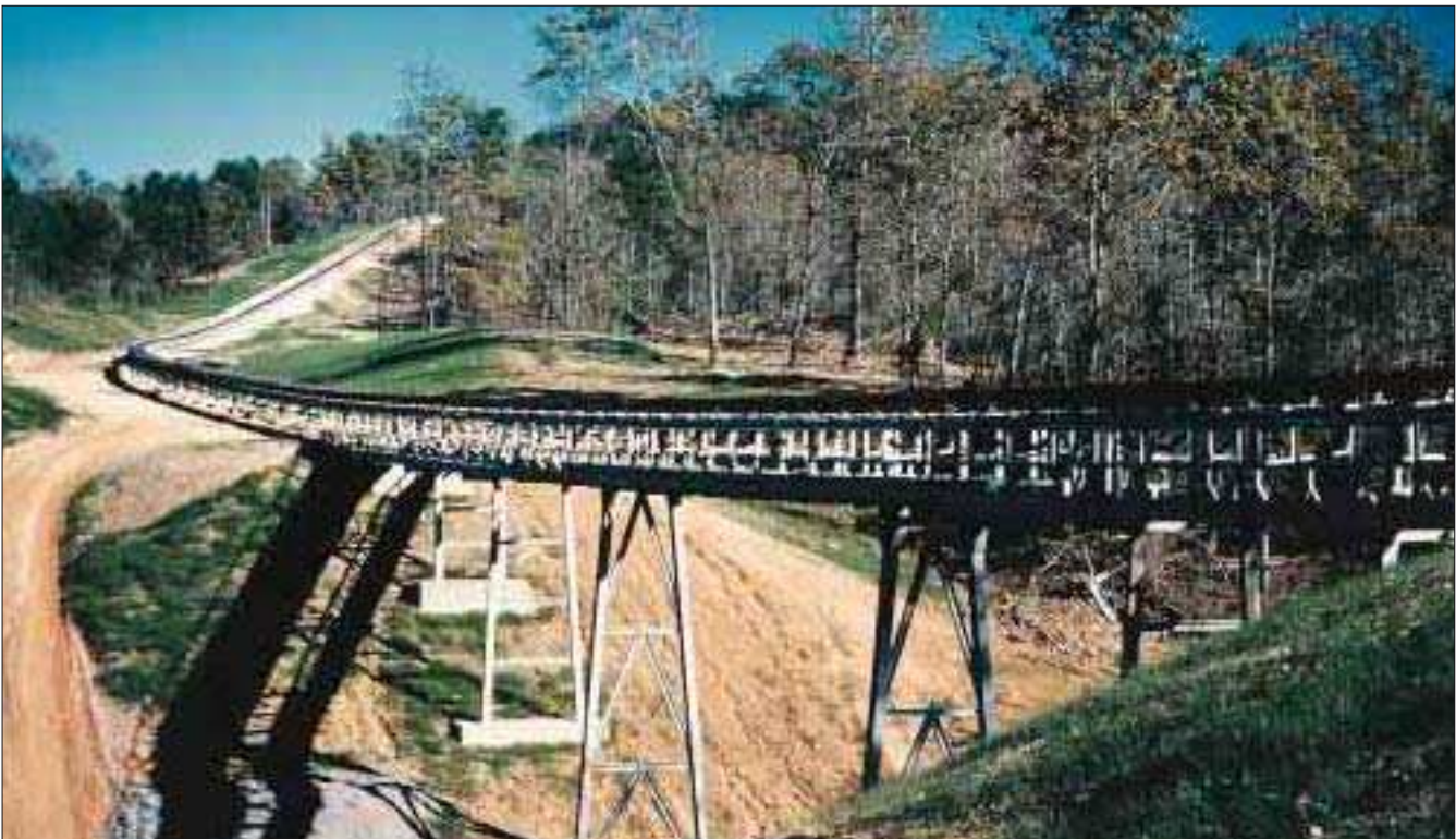
Horizontally curved troughed belt conveyor for the transport of limestone from the quarry to the cement factory
