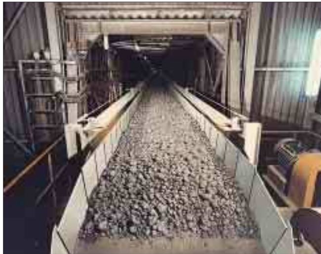
Apron conveyor for the transport of clinker with non-contacting overlapping cells
