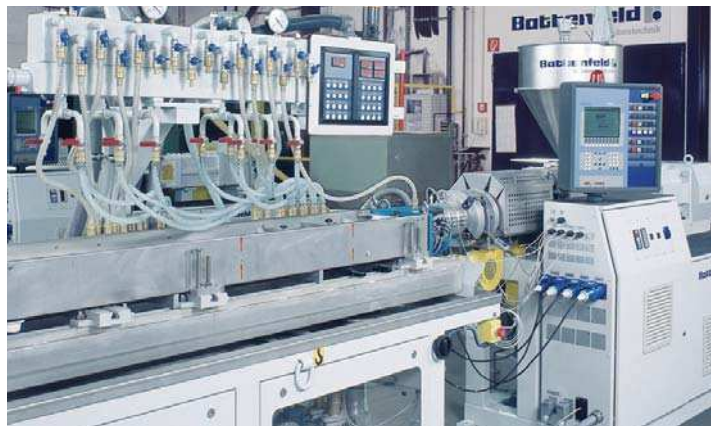
Calibration table for small profiles (K 162)
