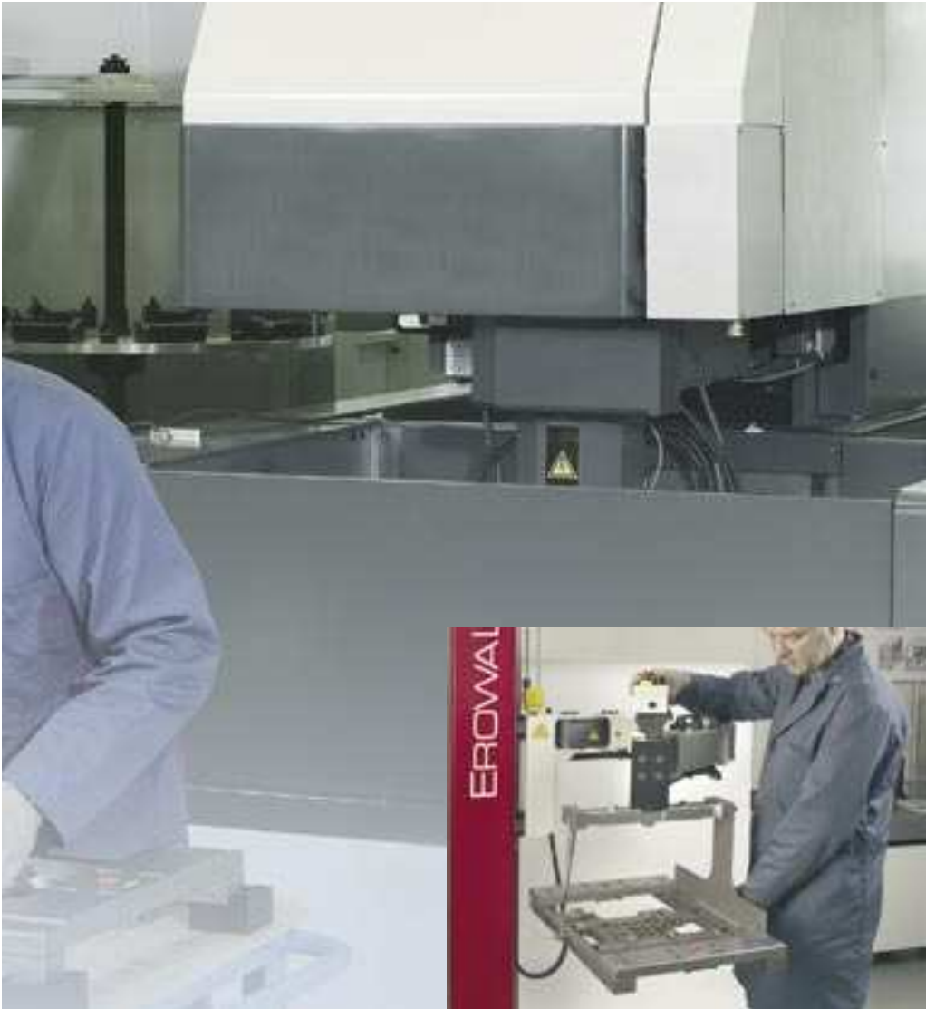
Loading Robot – for more machine autonomy at night and on weekends.
