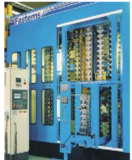
Automated Central Tool Storage, CTS, with Tool Gantry enables location of all spare tools in a central magazine and automates tool change to MC magazines from Central Tool Storage.
