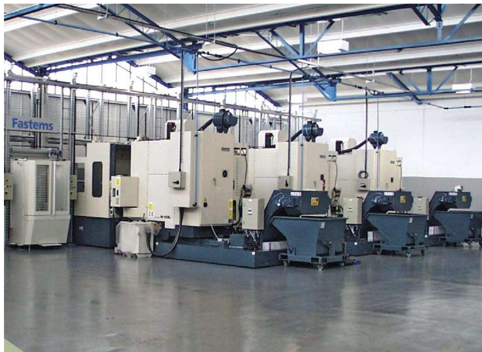
Standard FPM-LD with two LFS loading stations.
