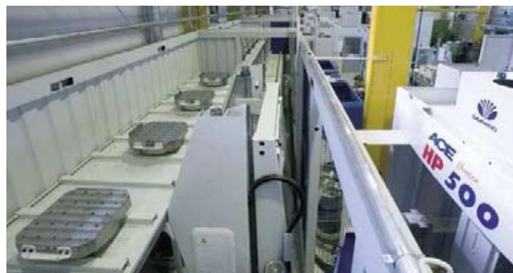
Three FPC-750 basic units in line.
