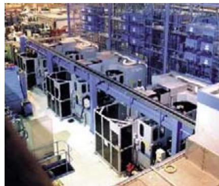
Automated Central Tool Storage, CTS, with Tool Gantry enables location of all spare tools in a central magazine and automates tool change to MC magazines from Central Tool Storage.
