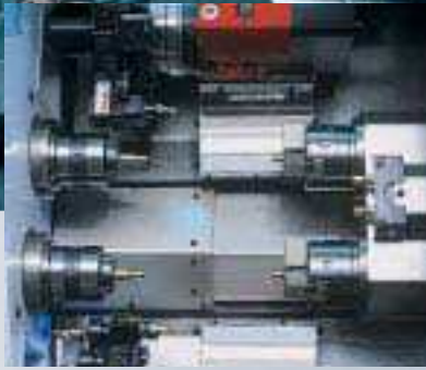
Twice as nice: 2 main spindles, 2 counter-spindles, 2 tool turrets for 2 fully machined finished parts
