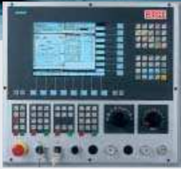
SINUMERIK 840D with EMCO specials – i.e. function buttons with LEDs as backlighting
