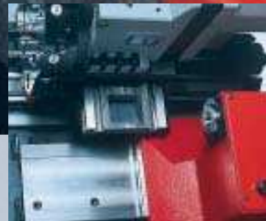
The standard tailstock is positioned manually. The quill is program-controlled (120 mm (4.7") stroke).
