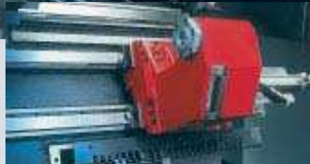
The automatic tailstock is freely programmable and can be positioned within the 510 mm (20.1") stroke.
