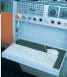
Hinged PC keyboard. Ergonomics all the way a major benefit, especially when most programming is done at the machine.
