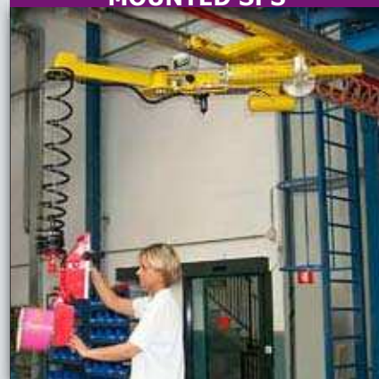
OVERHEAD TROLLEY MOUNTED SPS
